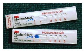
MonitorMark<sup>TM</sup> Time Temperature Indicators add an important temperature exposure measure that extends beyond your plant to your customers' delivery dock.
