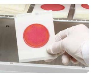
3M Petrifilm Aqua Plates are sample-ready media that replace conventional agar, petri dishes, media pads and disposable filter funnels used in the microbial testing of bottled water.
