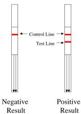
At least one line, the Control Line, should always develop. A red line in this position indicates that the strip is functioning properly. If the test strip displays 2 red lines, the test is complete and the sample is positive for Salmonella.
