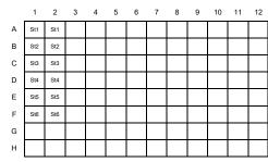
Example plate layout (example for a 6 point standard curve)
