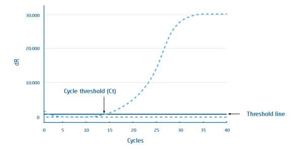
Amplification plot with the number of PCR cycles is shown on the x-axis, and the background subtracted fluorescence from the amplification reaction is shown on the y-axis. The threshold line is used to find the Ct value, where it intersects the amplification curve. Ct is optimally determined in the early exponential phase, when the fluorescence starts increasing due to PCR amplification. The threshold line is calculated automatically by the instrument giving in this example a Ct value of 14.
