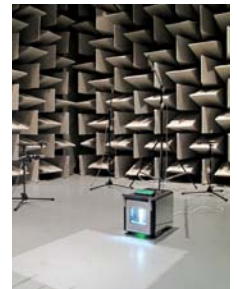
ISO 3744 acoustic test
