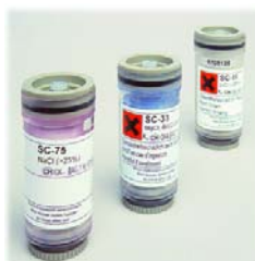
Novasina SC Humidity check for industrial air application.
