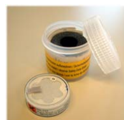
Novasina SAL-T humidity check for water activity application.
