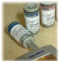
Humidity check on a HygroMate handheld instrument
